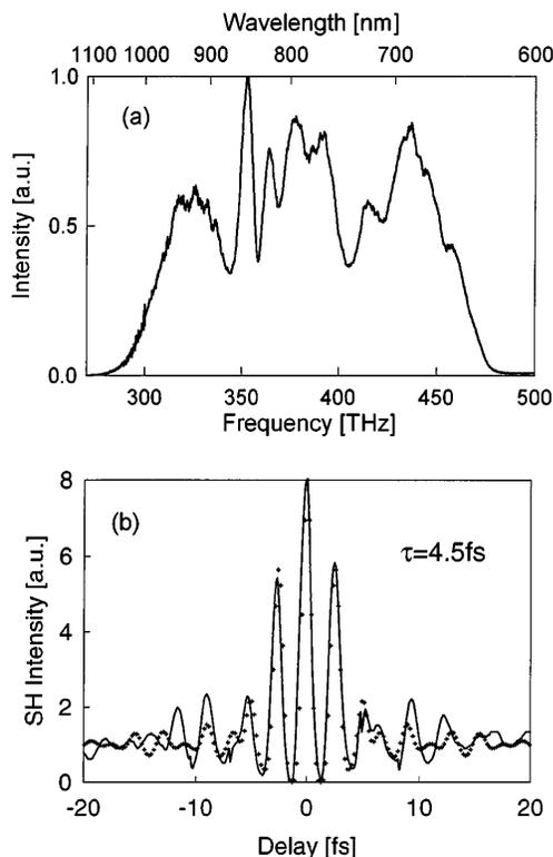
Fig. 2. (a) Spectral broadening in krypton at  $p = 2.1$  bars and  $P_0 = 2$  GW. A low-intensity pedestal ( $\sim 1\%$  of the peak) extends below 600 nm. (b) Measured (solid curve) and calculated (crosses) autocorrelation trace; an evaluation of the pulse duration (FWHM) is also given.
