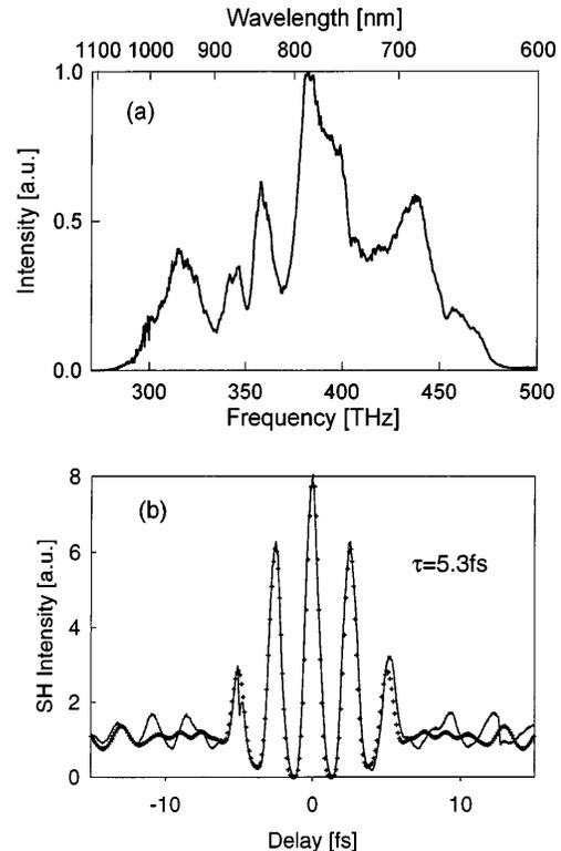
Fig. 1. (a) Spectral broadening in argon at  $p = 3.3 \text{ bars}$  and  $P_0 = 4 \text{ GW}$ . A low-intensity pedestal ( $\sim 1\%$  of the peak) extends below 600 nm. (b) Measured (solid curve) and calculated (crosses) autocorrelation trace; an evaluation of pulse duration (FWHM) is also given.
