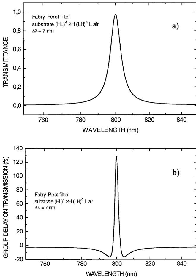
**Fig. 1.** **a** Computed transmittance and **b** group delay on the transmission of a thin film realization of a Fabry-Perot type interference filter having the structure of substrate (HL)<sup>4</sup> 2H (LH)<sup>4</sup> L air, where H and L denote quarterwave thick layers of the high ( $n_H = 2.31$ ) and low ( $n_L = 1.45$ ) refractive index materials at the central wavelength of 800 nm
