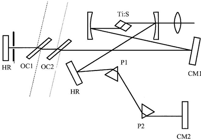
**Fig. 3.** Schematic sketch of the cavity setup
