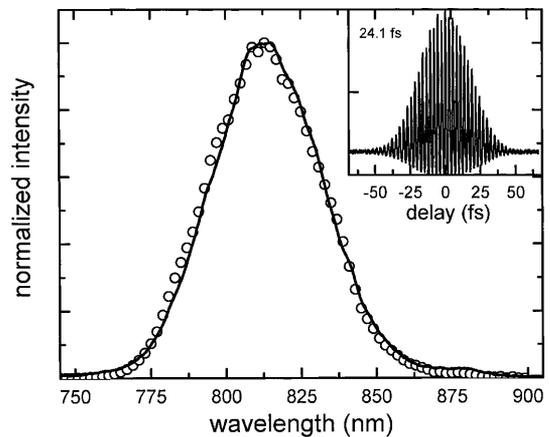
**Fig. 6.** Pulse spectrum from the long wave OC: measured (solid line) and calculated by multiplying the intracavity spectrum by the reflectivity of the long wave OC (circles). Inset: respective fringe resolved autocorrelation trace
