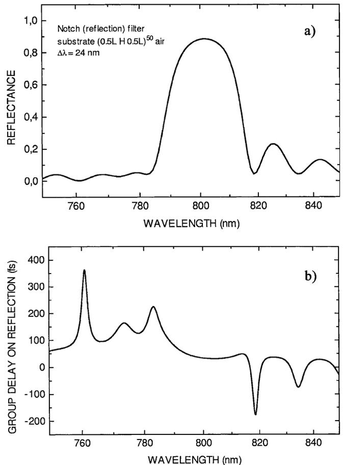
**Fig. 2.** **a** Computed reflectance and **b** group delay on reflection of a thin film realization of a typical realization of a (reflective) notch interference filter having the structure of substrate (0.5L H 0.5L)<sup>50</sup> air, where H and L denote quarterwave thick layers of the high ( $n_H = 1.5$ ) and low ( $n_L = 1.45$ ) refractive index materials at the central wavelength of 800 nm
