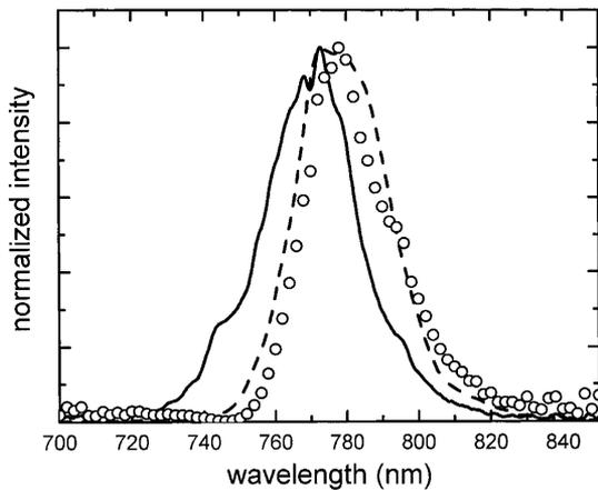
**Fig. 7.** Single-color operation without short wave OC: the measured extracavity spectrum (*dashed line*) is well reproduced (*circles*) by multiplying the intracavity spectrum (*solid line*) by the reflectivity of long wave OC
