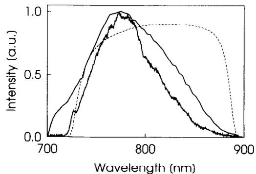
Fig. 4. The dashed line indicates the overall transmittivity of the system, which narrows the  $\approx 100 \text{ nm}$  broad seed spectrum (upper solid line) to  $\approx 70 \text{ nm}$  (lower solid line).
