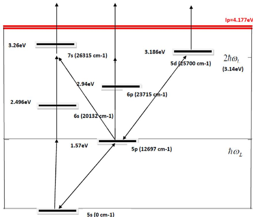
Fig. 4. The relevant energy levels of the Rb atom along with the two-photon excitation and three-photon ionization scheme.
