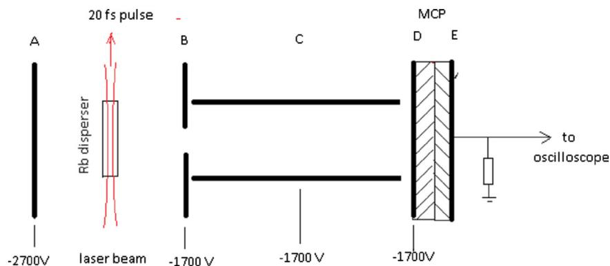
Fig. 1. The scheme of the experimental setup.
