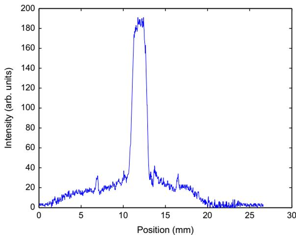
Fig. 3. The shape of the Rb atomic beam above the opening slit.
