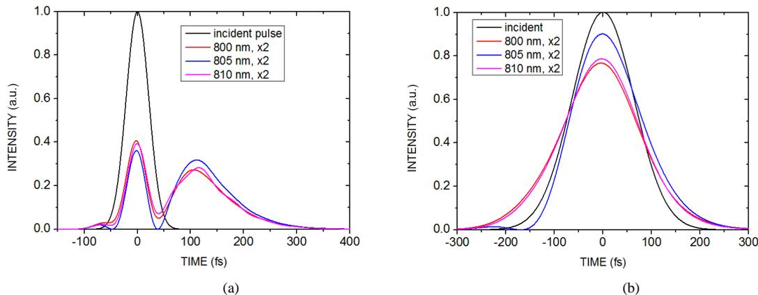
**Fig. 3** Calculated intensity vs. time functions of transform limited (a) 50 fs and (b) 150 fs pulses being reflected on an ultra-broadband dielectric mirror 508-519 (Newport Corp.) for s-polarized light at 45° AOI.
