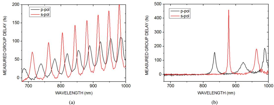
Fig. 2 Measured group delay vs. wavelength functions of ultra-broadband dielectric mirrors (a) CODE: 508-519 (Newport Corp.) and (b) BB1-E03 (Thorlabs Inc.)
